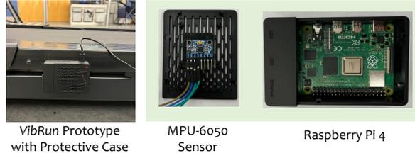
Fig. 7. Hardware implementation of VibRUN showing components within the case and connections between the components.
