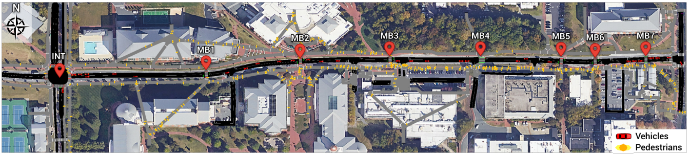
Fig. 1: The Craver Road corridor with an intersection (INT) that contains one primary traffic signal and four signalized crosswalks, along with seven midblock signalized crosswalks (MB1–MB7) that control pedestrian–vehicle interactions.
